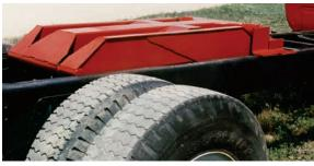
Hoist mounts low between the frame, meaning no notching crossmemebers under dump body.
